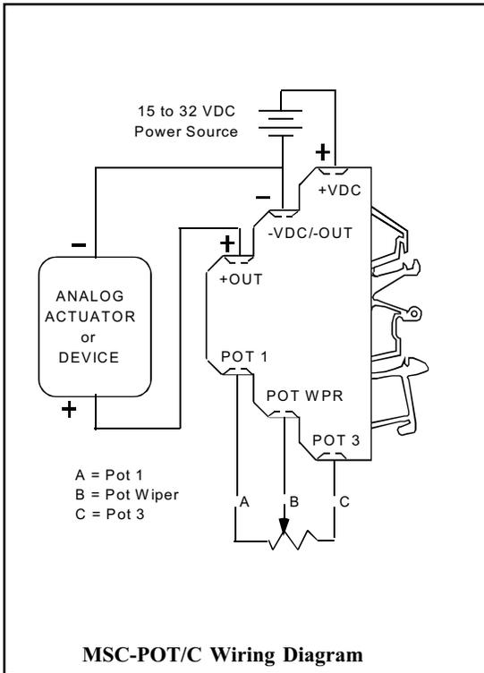
**Warning:** Initial power-up requires a minimum of 15Vdc and a maximum of 32 Vdc. Any voltage outside this range will cause damage to the unit. When installing or servicing the unit, take precautionary steps in preventing any electrostatic discharge to the unit.
